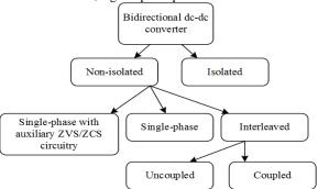
Fig.1. Simplified classification of the bidirectional dc-dc power converters.
