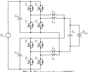
Fig. 5. Floating interleaved NBDC.
